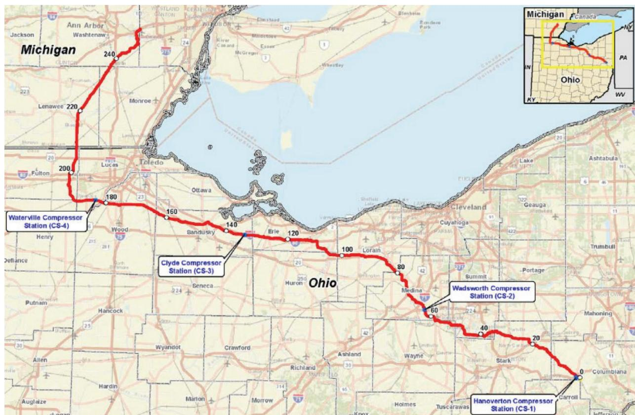
**FIGURE 1.** Nexus Pipeline Proposed Route. This map shows the proposed 256-mile Nexus Pipeline route, transecting northern Ohio and southeastern Michigan, terminating at the Dawn Hub in Ontario, Canada. The compressor stations, where the pipeline pressure is maintained, are also identified. Note, the Maumee River Crossing is near mile marker 180 and in close proximity to the Waterville Compressor Station.
