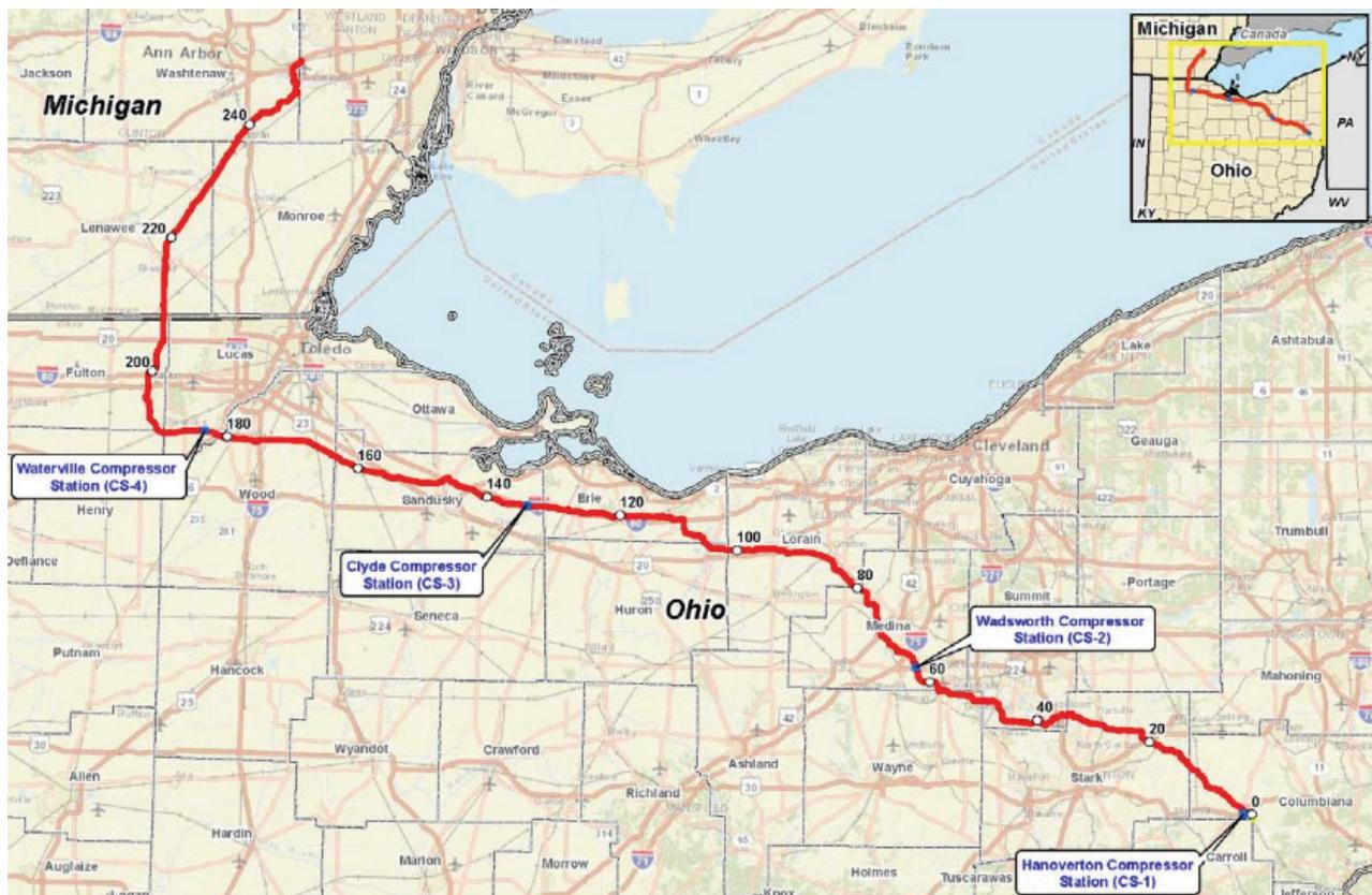
**FIGURE 1.** Nexus Pipeline Proposed Route. This map shows the proposed 256-mile Nexus Pipeline route, transecting northern Ohio and southeastern Michigan, terminating at the Dawn Hub in Ontario, Canada. The compressor stations, where the pipeline pressure is maintained, are also identified. Note, the Maumee River Crossing is near mile marker 180 and in close proximity to the Waterville Compressor Station.
